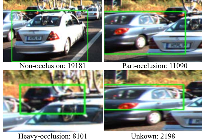
Fig. 1. Sample numbers of different occlusion levels are collected based on the KITTI dataset. Occlusion happens all the time in real traffic, such as traffic jams, narrow roads, the parallel cars changing lanes. We categorize the level of occlusion into four classes: non-occlusion, part-occlusion, heavy-occlusion, and unknown.
